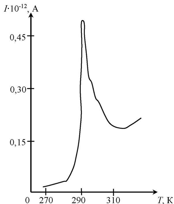
Figure 2 – Curve of the TSC current of a non-degraded LED at a heating rate of  $\beta = 0,112$  K/s
