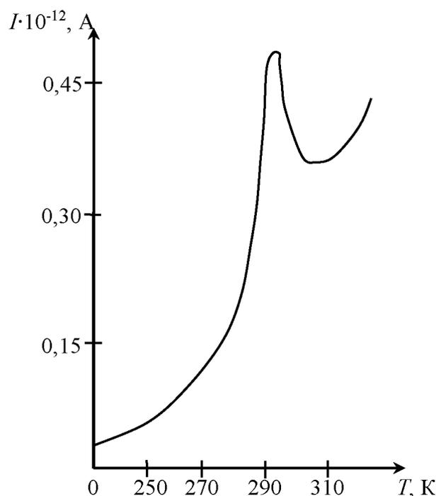
Figure 3 – Curve of the current TST of the LED after degradation at heating rate of  $\beta = 0,09$  K/s
