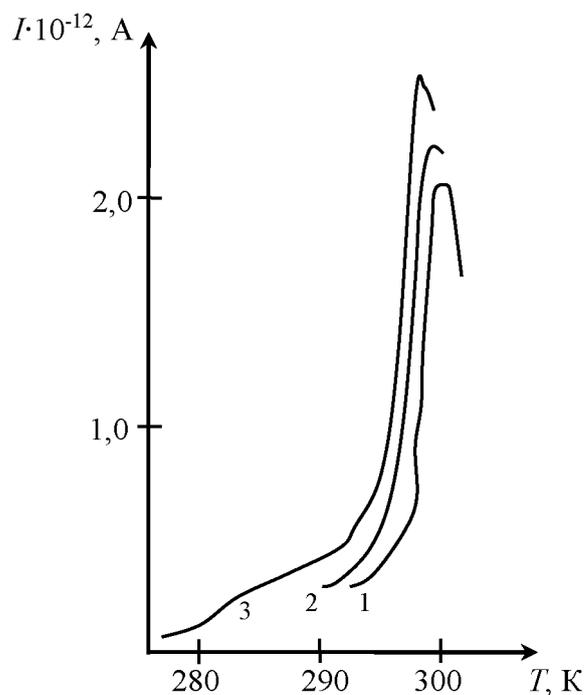
Figure 1 – Illustration of thermal cleaning of the TSC light emitted diode peak based on  $GaAlAs$  at a heating rate of  $\beta = 0,25$  K/s
